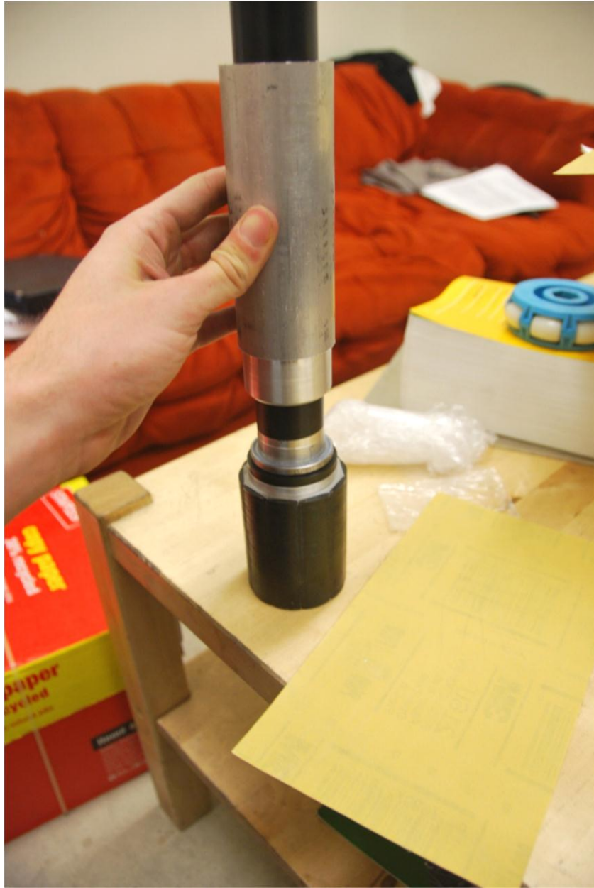
Figure 3.4: Installation tool for bearings.
