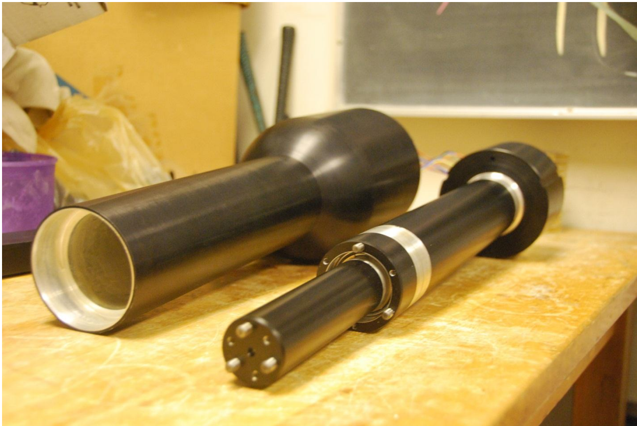
Figure 3.5: Assembled inner/outer shafts and outer housing.
