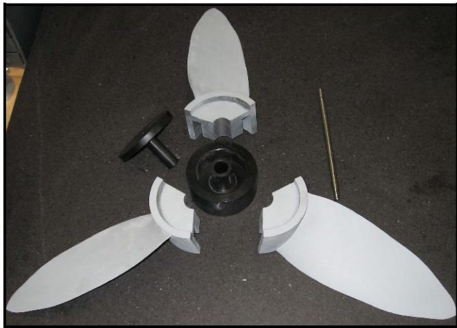
Figure 6. Case study: Propeller design for a high-drag Autonomous Underwater Vehicle.
